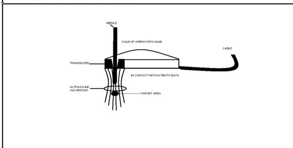
Fig 1. Cross section of novel ultrasound probe
